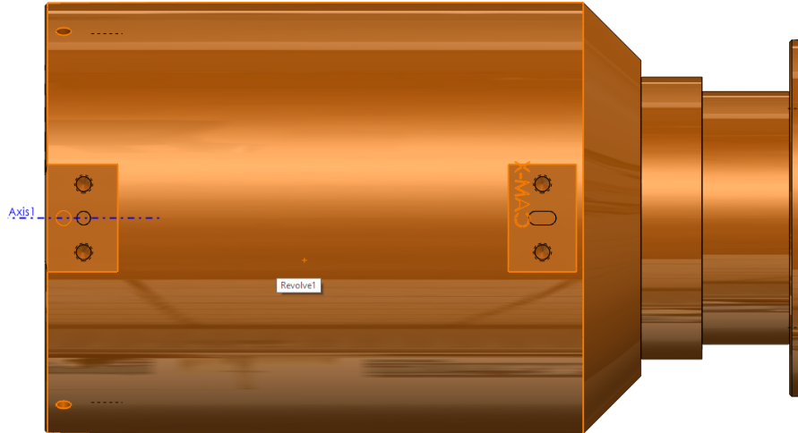
Figure 12: Bottom view of one of the camera barrels showing the locations of the hole and slot to receive the pins in the mounting bracket with threaded holes for the m4 screws to secure the barrels to the mounts.
