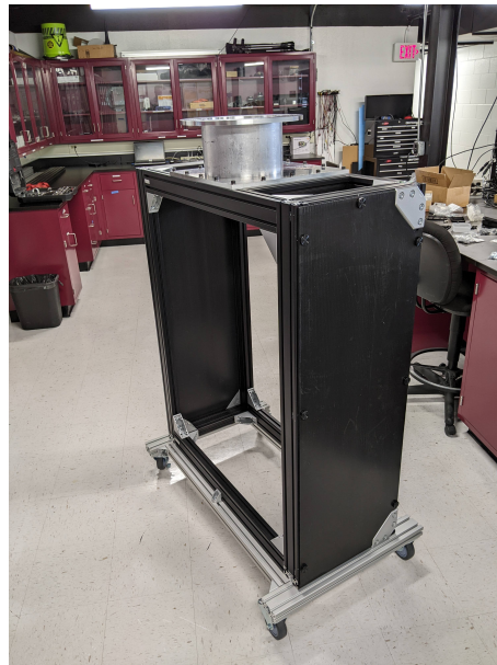
Figure 11: Temporary extruded frame with two of the side panels attached. A removable cart (silver extrusions) allows ETSI to be rolled around the lab, or into position when mounting to the telescope.
